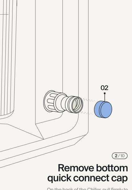
On the back of the Chiller, pull firmly to remove the cap on water in port.
