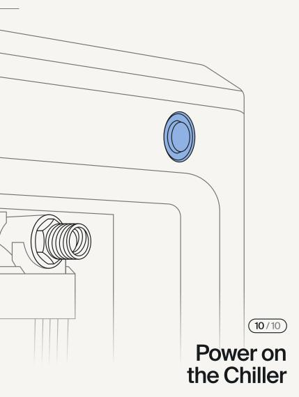
Connect Chiller to power and hold the back button for 3 seconds to turn on.
