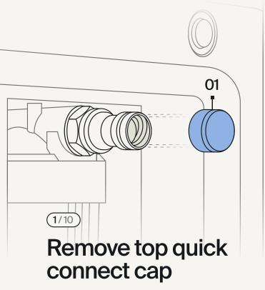
On the back of the Chiller, pull firmly to remove the cap on water out port.
